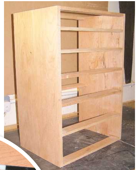
▲ Pic.6 Here's the assembled carcass; note the single mid-rail at the back
